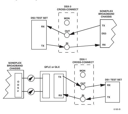
Figure 510-1. Test Setup
